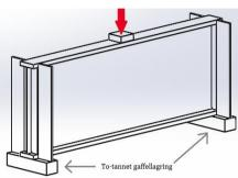
Fig 9. Simply supported, end-fork stabilized plate-girder All steel: S355
