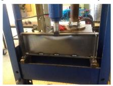
Fig 10. Beam with no internal stiffeners, Configuration I, after web buckling
