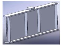
Fig 6. Plate Girder with two stiffeners spaced at 182 mm each side of web and centered om point of load application
