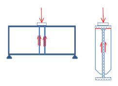
Fig 1. Transfer of point-load through web-stiffener to girder-web
