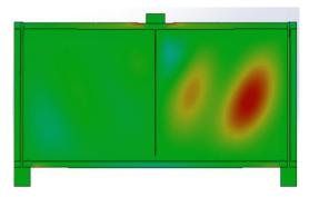
Fig 17.Initial buckling with one interior stiffener ea.s. of the web
